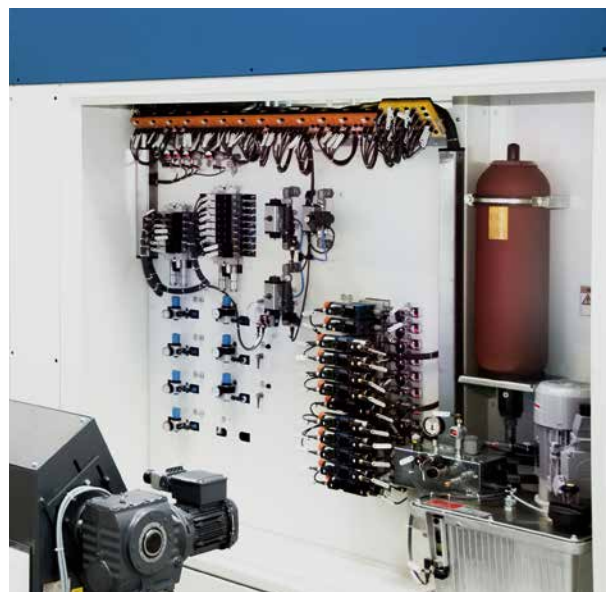
Fluid cabinet (side view of the machine)
