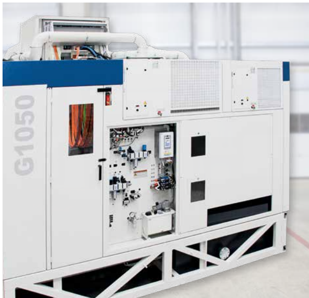
Fluid cabinet (rear view of the machine)
